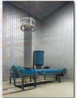
Test transformer, coupling capacitor and impulse voltage lead-in bushing and 1,500kV impulse voltage generator
