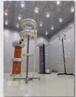
3,000kV impulse voltage generator and 1,000kV power frequency withstand voltage and partial discharge test system
