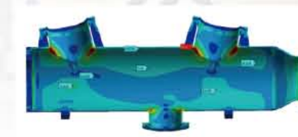
Enclosure mechanical strength analysis
