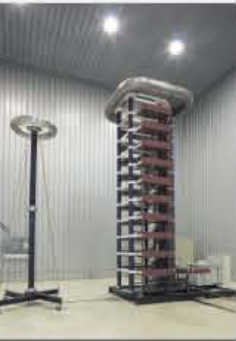
Test transformer, coupling capacitor and impulse voltage lead-in bushing and 1,500kV impulse voltage generator
